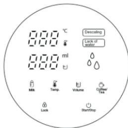
**Lock** button: press it about 3-5 seconds to unlock, lock without any act within 10-15 seconds, you can lock the screen free by press **Lock** button.
